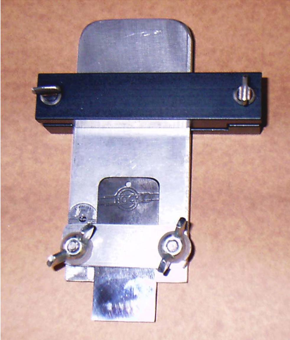
Self Squaring Tool Clamp with adapter to hold a small plane iron.
